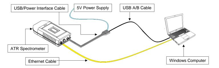
When you run a wired connection please make sure that you connect the spectrometer as follows:
