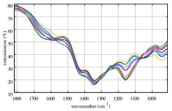
Mid-infrared absorption spectra of a typical marine engine oil at different points during the lifetime of the oil. Note the visible changes in the spectra which are related to specific oil degradation effects.
