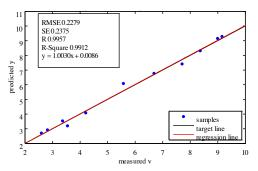
The Total Base Number (TBN) has been calculated from the measured absorption spectra using the SphinxSuite software module. The plot compares the TBN obtained from analysing the mid-infrared absorption spectra to the TBN obtained from the same oil sample in an accredited oil analysis laboratory. The correlation between the results is exceptional.
