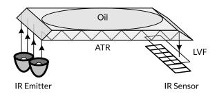
If now a sample is placed on top of the ATR crystal the refractive index of that sample is different to that of air resulting that the light penetrates which each bounds a certain distance into the sample before it is reflected back into the ATR crystal (evanescent waves). Which each bounce certain wavelength of the light are absorbed by the sample sitting on top of the ATR crystal.
