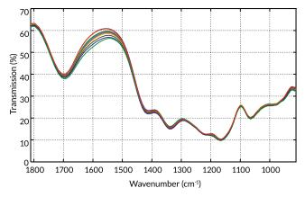
Mid-IR spectroscopy is able to provide information (qualitatively and quantitatively) about the three different aging mechanism. By a detailed analysis of the mid-infrared absorption spectrum of an oil sample the oil condition can be characterised and specific degradation mechanism can be identified and analysed.
