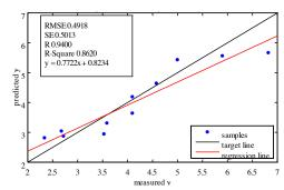
The i-pH value has been calculated from the measured absorption spectra using the SphinxSuite software module. The plot compares the i-pH values obtained from analysing the mid-infrared absorption spectra to the i-pH values obtained from the same oil samples in an accredited oil analysis laboratory. The data indicate that the oil reference data obtained from the oil laboratory should be checked as they indicate a saturation effect (systematic error of titration technique for i-pH value).
