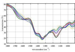
Mid-infrared absorption spectra of a typical biogas engine oil at different points during the lifetime of the oil. Note the visible changes in the spectra which are related to specific oil degradation effects.
