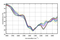
Mid-infrared absorption spectra of a typical biogas engine oil at different points during the lifetime of the oil. Note the visible changes in the spectra which are related to specific oil degradation effects.
