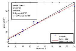
The oil oxidation has been calculated from the measured absorption spectra using the SphinxSuite software module. The plot compares the oil oxidation levels obtained from analysing the mid-infrared absorption spectra to the oxidation levels obtained of the same oil sample in accredited oil analysis laboratory. The correlation between the results is exceptional.
